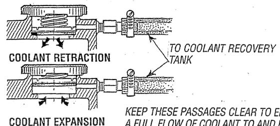
KEEP THESE PASSAGES CLEAR TO ENSURE A FULL FLOW OF COOLANT TO AND FROM THE COOLANT RECOVERY TANK (A PIPE CLEANER WORKS WELL)
