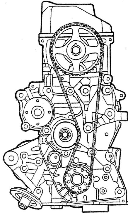
5. Turn the crankshaft twice in the normal rotating direction (clockwise) and check that the timing marks are correctly aligned.
