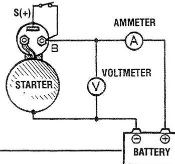
**CAUTION:** Use thick wires as much as possible and tighten every terminal securely. This is a solenoid shift-type starter which makes a rotating sound louder than that of a direct-drive type starter. When detecting starter rotation at the pinion tip, be careful not to come in contact with the pinion gear when it protrudes.
