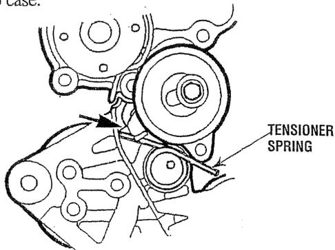
3. Grip the other tensioner spring projection and fit it onto the oil pump case lug as shown in the illustration. Move the timing belt tensioner in the direction shown and temporarily tighten the bolt.
