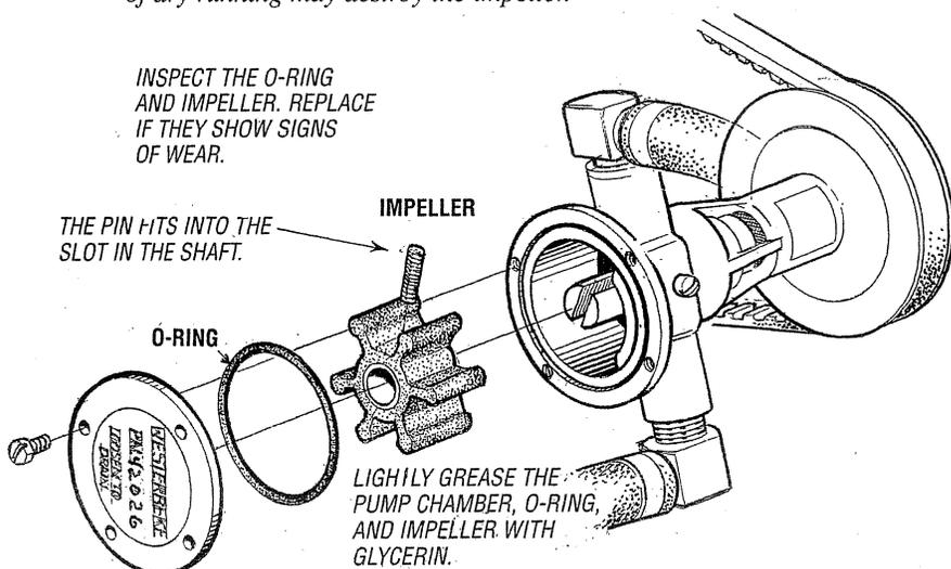
**CAUTION:** If any of the blades have broken off the impeller, they must be located to prevent blockage in the cooling circuit. They often can be found in the heat exchanger
