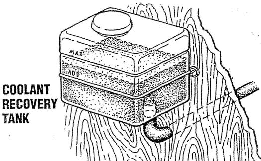
**NOTE:** Periodically check the condition of the manifold pressure cap, its rubber seals and the vacuum return valve. Ensure the passage from the filler neck to the recovery tank connection is kept clear.
