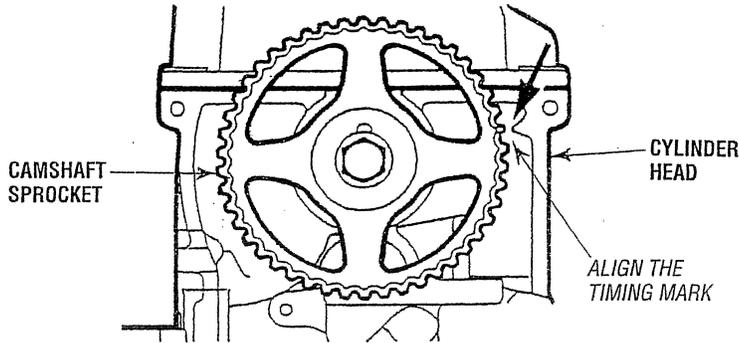
1. Align the camshaft timing mark with the timing mark on the cylinder head.
