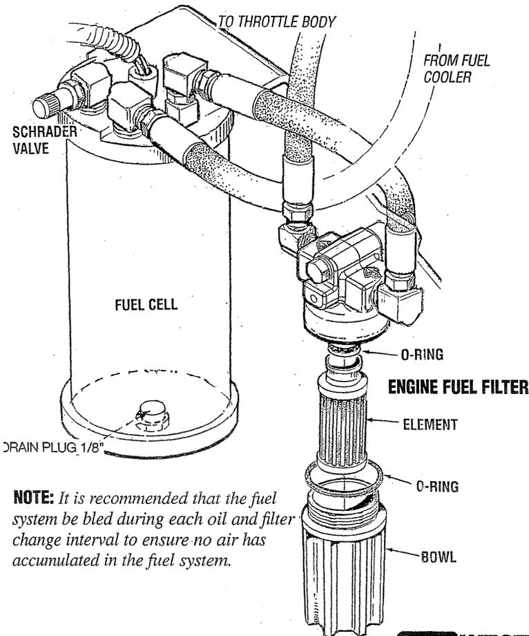
**NOTE:** It is recommended that the fuel system be bled during each oil and filter change interval to ensure no air has accumulated in the fuel system.
