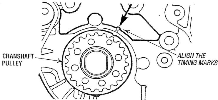
2. Align the crankshaft timing mark with the timing mark on the front case.
