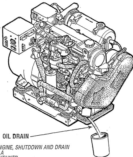
WARM THE ENGINE, SHUTDOWN AND DRAIN THE OIL INTO A SUITABLE CONTAINER
