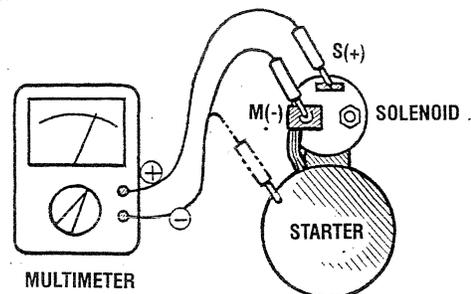
**NOTE:** Disconnect the wire from terminal M.
