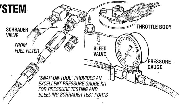
8. Remove the pressure gauge set, and cap all Schrader valves.
