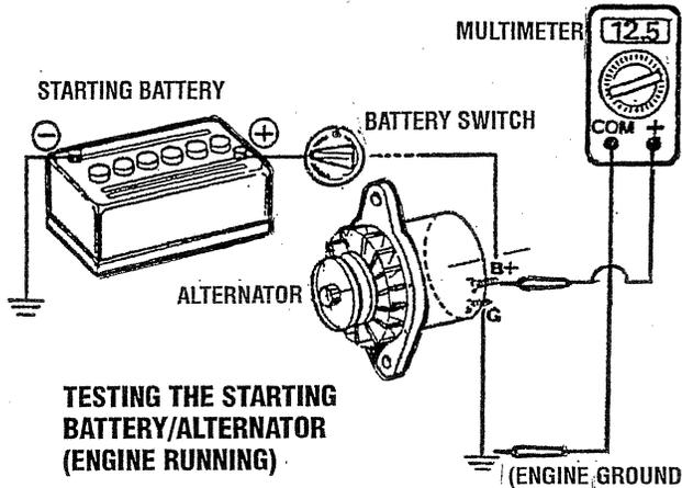
8. Start the engine again. Check the voltage between the alternator output and ground. The voltage reading for a properly operating alternator should be between 13.5 and 14.5 volts. If your alternator is over- or under-charging, have it repaired at a reliable service facility.
